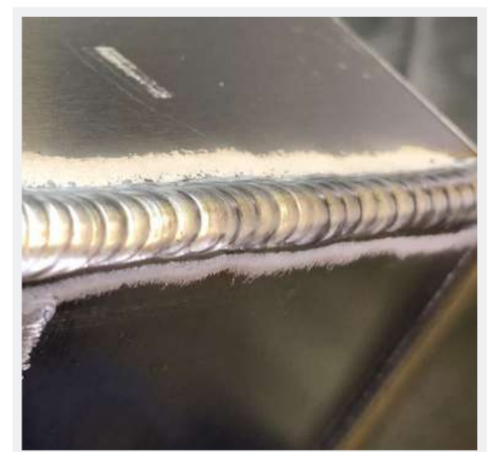
An example of a strong and visually pleasing aluminium TIG weld
