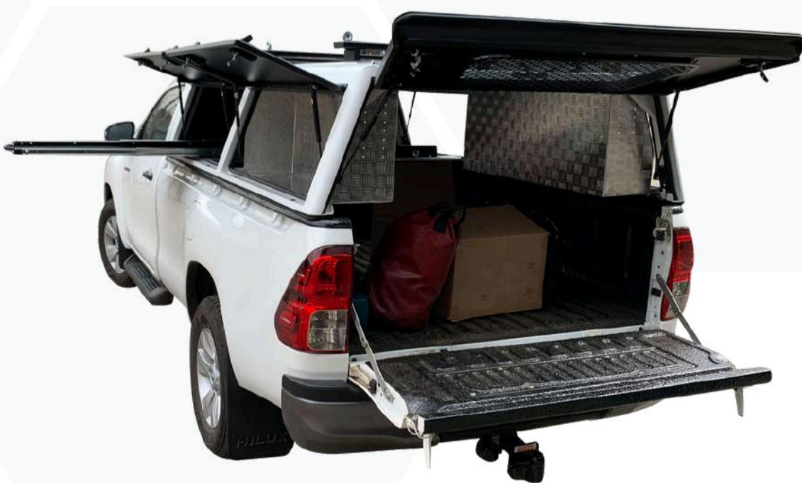
Telescopic slide for access to additional storage as well as rear mounted storage boxes
